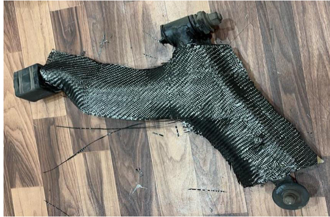
Fig. Carbon Fiber sheet cut according to the LCA dimensions
