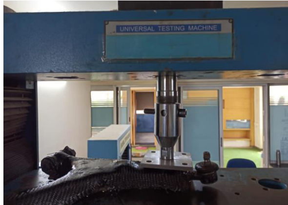
Fig. Specimen under Compression test using UTM
